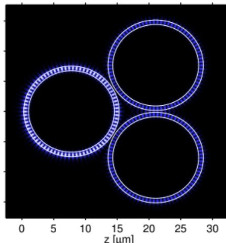
$$\begin{aligned}\lambda_r &= 1.56234 \mu\text{m}, \\ Q &= 1.0 \cdot 10^5, \\ \Delta\lambda &= 1.5 \cdot 10^{-5} \mu\text{m}.\end{aligned}$$
