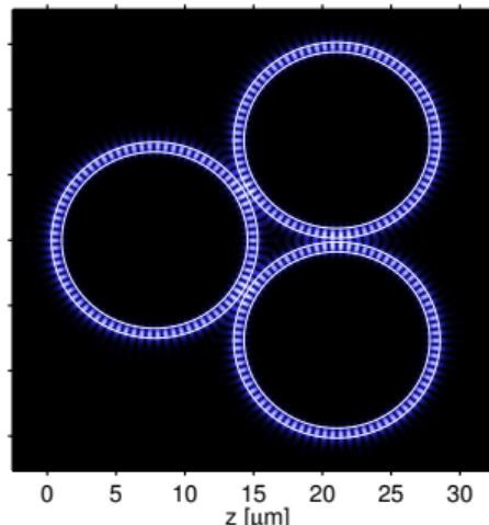
$$\begin{aligned}\lambda_r &= 1.56946 \mu\text{m}, \\ Q &= 1.3 \cdot 10^5, \\ \Delta\lambda &= 1.1 \cdot 10^{-5} \mu\text{m}.\end{aligned}$$
