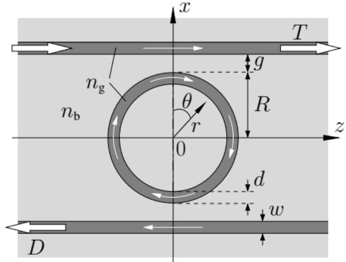
TE,  $R = 7.5 \mu\text{m}$ ,  $w = 0.6 \mu\text{m}$ ,  $d = 0.75 \mu\text{m}$ ,  $g = 0.3 \mu\text{m}$ ,  $n_g = 1.5$ ,  $n_b = 1.0$ ,  $\lambda \approx 1.55 \mu\text{m}$ .
