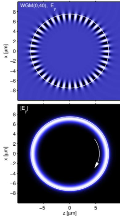
$$\begin{aligned}\lambda_r &= 1.56514 \text{ } \mu\text{m}, \\ Q &= 8.2 \cdot 10^5, \\ \Delta\lambda &= 1.9 \cdot 10^{-6} \text{ } \mu\text{m}.\end{aligned}$$
