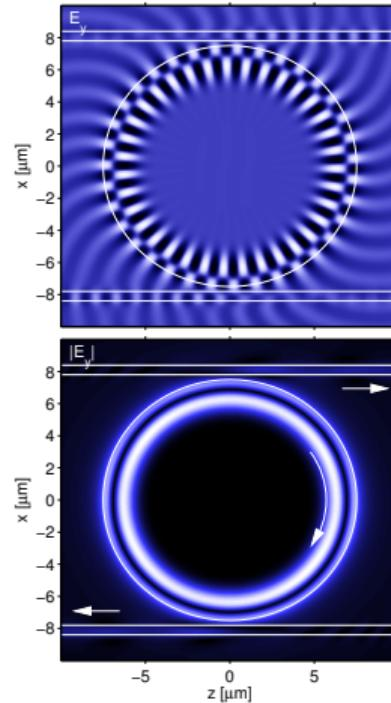
$$\begin{aligned}\lambda_r &= 1.57320 \text{ } \mu\text{m}, \\ Q &= 1.1 \cdot 10^3, \\ \Delta\lambda &= 1.4 \cdot 10^{-3} \text{ } \mu\text{m}.\end{aligned}$$
