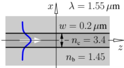
Basis element: forward TE<sub>0</sub> mode,  $f_0 = 1$ ,
