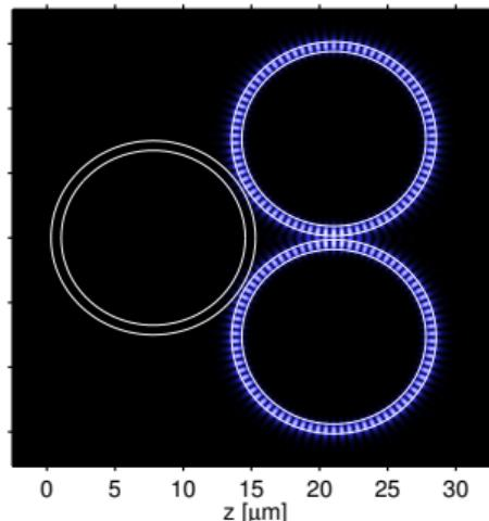
$$\begin{aligned}\lambda_r &= 1.56715 \mu\text{m}, \\ Q &= 1.2 \cdot 10^5, \\ \Delta\lambda &= 1.3 \cdot 10^{-5} \mu\text{m}.\end{aligned}$$
