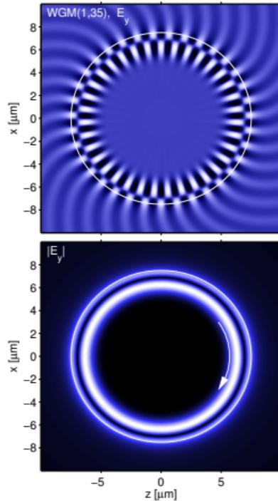
$$\begin{aligned}\lambda_r &= 1.57444 \text{ } \mu\text{m}, \\ Q &= 1.6 \cdot 10^3, \\ \Delta\lambda &= 9.2 \cdot 10^{-4} \text{ } \mu\text{m}.\end{aligned}$$
