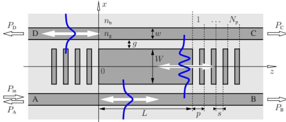
$$\begin{aligned} n_g &= 1.60, n_b = 1.45, \\ w &= 1.0 \mu\text{m}, g = 1.6 \mu\text{m}, \\ W &= 9.955 \mu\text{m}, \\ L &= 79.985 \mu\text{m}, \\ p &= 1.538 \mu\text{m}, \\ s &= 0.281 \mu\text{m}, \\ N_p &= 40. \end{aligned}$$
