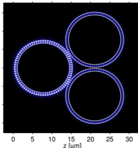
$$\begin{aligned}\lambda_r &= 1.56714 \mu\text{m}, \\ Q &= 0.9 \cdot 10^5, \\ \Delta\lambda &= 1.7 \cdot 10^{-5} \mu\text{m}.\end{aligned}$$
