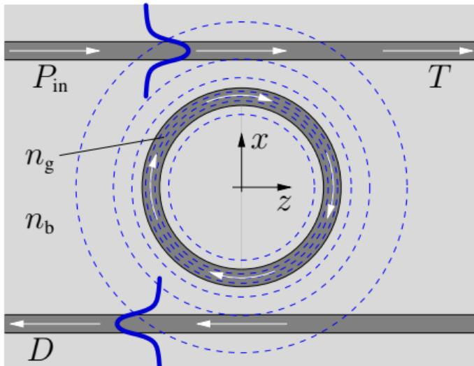
$$\left\{ \omega_j^c, \left( \frac{\tilde{\mathbf{E}}}{\tilde{\mathbf{H}}} \right)_j^c(x, z) \right\}, \quad P_{\text{in}}(\omega) \text{ given: } T(\omega), D(\omega) = ?$$
