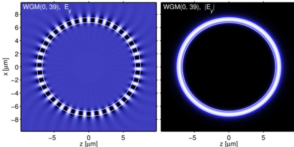
TE,  $R = 7.5 \mu\text{m}$ ,  $d = 0.75 \mu\text{m}$ ,
