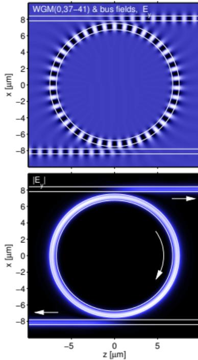
$$\begin{aligned}\lambda_r &= 1.5637 \text{ } \mu\text{m}, \\ Q &= 1.1 \cdot 10^5, \\ \Delta\lambda &= 1.4 \cdot 10^{-5} \text{ } \mu\text{m}.\end{aligned}$$
