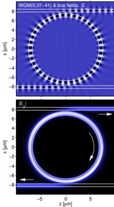
$$\begin{aligned}\lambda_r &= 1.56219 \mu\text{m}, \\ Q &= 4.3 \cdot 10^2, \\ \Delta\lambda &= 3.7 \cdot 10^{-3} \mu\text{m}.\end{aligned}$$
