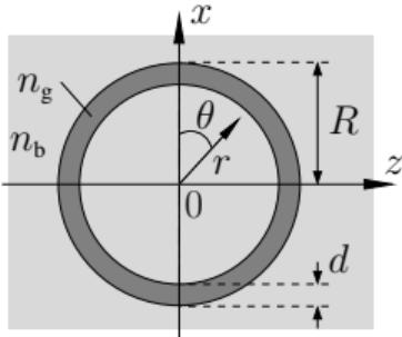
TE,  $R = 7.5 \mu\text{m}$ ,  $d = 0.75 \mu\text{m}$ ,  $n_b = 1.0$ .
