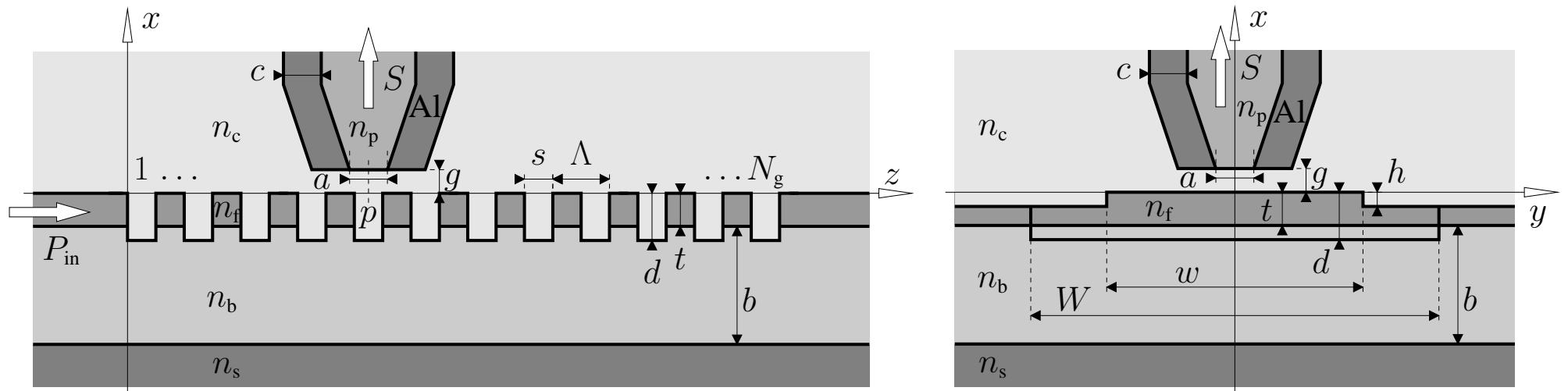
**Sample:** Rib waveguide with a series of deep, rectangular slits,
