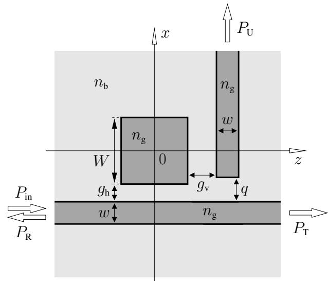
$W = 1.786 \mu\text{m}$ ,  $w = 1.0 \mu\text{m}$ ,
