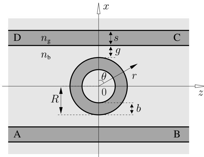
$R = 50 \mu\text{m}$ ,  $b = s = 1.0 \mu\text{m}$ ,  $g = 0.9 \mu\text{m}$ ,
