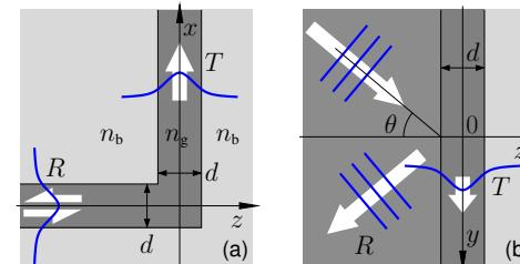
$$n_g = 3.4, \\ n_b = 1.45, \\ d = 0.25 \mu\text{m}, \\ \lambda = 1.55 \mu\text{m}, \\ \text{in: TE}_0.$$
