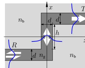
$$\begin{aligned} n_g &= 3.4, \quad n_b = 1.45, \\ d &= 0.25 \mu\text{m}, \quad h = 2.15 \mu\text{m}, \\ \lambda &= 1.55 \mu\text{m}, \quad \text{in: TE}_0. \end{aligned}$$
