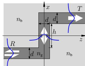
$$\begin{aligned} n_g &= 3.4, \quad n_b = 1.45, \\ d &= 0.25 \mu\text{m}, \quad h = 2.15 \mu\text{m}, \\ \lambda &= 1.55 \mu\text{m}, \quad \text{in: TE}_0. \end{aligned}$$
