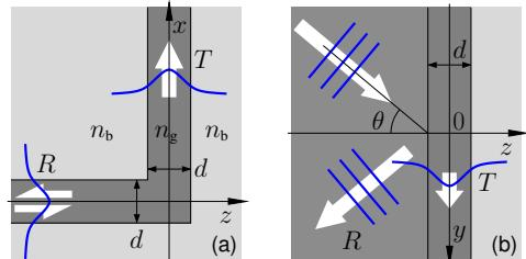
$$\begin{aligned}n_g &= 3.4, \\n_b &= 1.45, \\d &= 0.25 \mu\text{m}, \\&\\ \lambda &= 1.55 \mu\text{m}, \\ \text{in: } &\text{TE}_0,\end{aligned}$$
