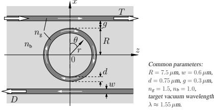
Given the analytical modes of the two bus cores and the bend mode(s) [8, 9, 10] supported by the curved waveguide profile that constitutes the cavity, one readily writes an ansatz for the time harmonic electromagnetic field, using the natural Cartesian and polar coordinates for the straight and curved waveguide elements.
