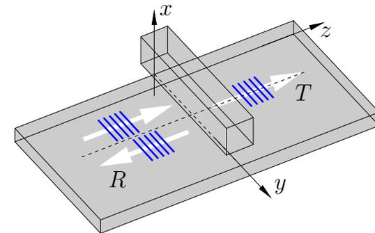
**An open dielectric resonator with a rectangular cavity**
