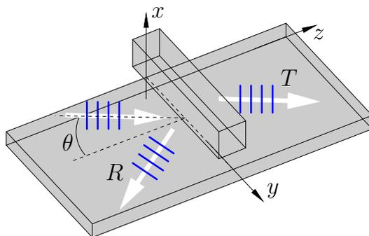
**An open rectangular dielectric optical cavity with unlimited Q**
