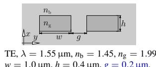
TE,  $\lambda = 1.55 \mu\text{m}$ ,  $n_b = 1.45$ ,  $n_g = 1.99$ ,  $w = 1.0 \mu\text{m}$ ,  $h = 0.4 \mu\text{m}$ ,  $g = 0.2 \mu\text{m}$ .
