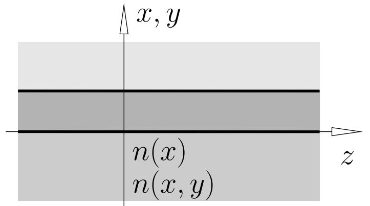
$$\mathcal{E}(x, y, z, t) = \text{Re} \mathbf{E}(x, y) e^{i\omega t - i\beta z}, \quad \mathcal{H}(x, y, z, t) = \text{Re} \mathbf{H}(x, y) e^{i\omega t - i\beta z}.$$
