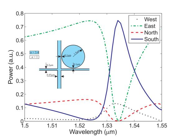
Spectrum of power leaving the window through the main modes of the guides at the four boundaries. East and west are fundamental modes; north and south are first order modes. The fundamental mode comes in from the left.
