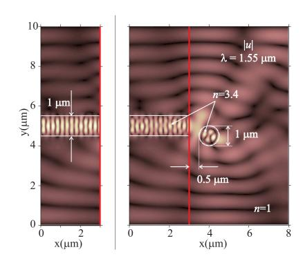
Fundamental mode of light comes in from the left. *Left pic-ture*: All information of the termination and obstacle is in the boundary. *Right picture*: Full finite element simulation, including termination and obstacle. The fields are nearly identical.
