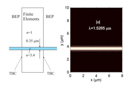
Light comes in as the fundamental mode from the left and leaves the right-hand boundary undisturbed.
