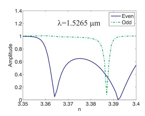
Amplitudes of even and odd Bloch modes on the right-hand boundary. The crystal is made of square pillars, n=3.4, 150 nm wide, with a pitch of 600 nm; the disk has a radius of 1.075  $\mu$ m, index 3.4.
