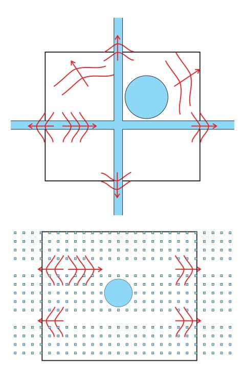
We want to have the boundary  $\partial\Omega$  of the domain  $\Omega$  be transparent for outgoing light, while taking into account waveguide structures leaving through the boundary and reflections caused by structures outside the domain.
