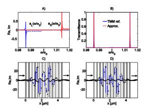
**Fig. 2.** A) Decomposition coefficients (frequency dependent weighting factors in the field template). B) Transmittance obtained from the field representation using QNMs (dashed) and TMM reference (continuous). C) and D): approximated field obtained from the field representation using QNMs (marker) and TMM reference for the frequency of transmission resonance (solid line) for  $\omega = Re(\omega_R)$ .
